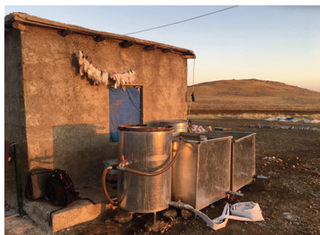
The three-tank, water-recycling flotation system.
