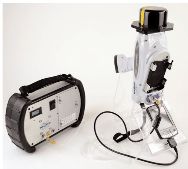
A Bruker Tracer III-SD analysis system (image courtesy of Bruker.com)
